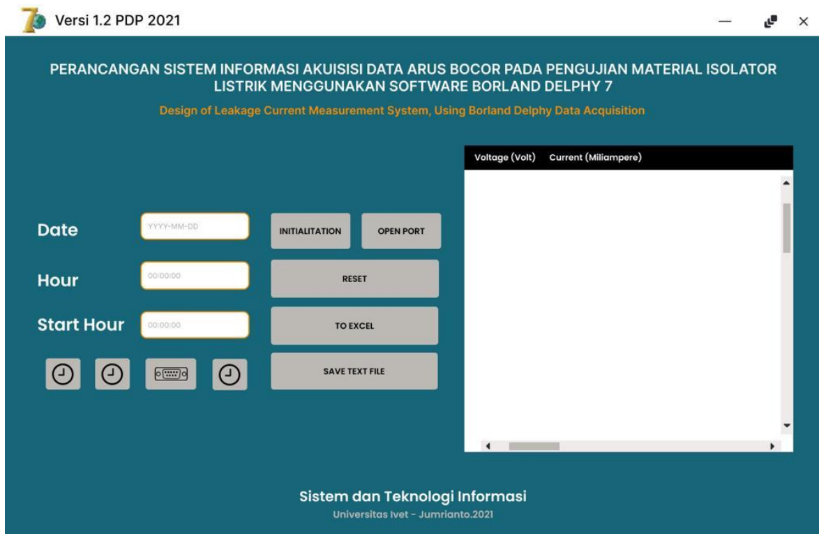
Gambar 1. Interface Software Pengujian Karakteristik Isolator Listrik
