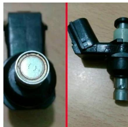
**Gambar 3.** Injector Racing 8 Hole
