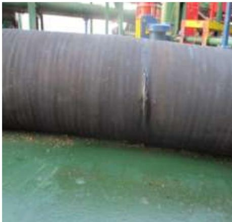
**Gambar 5.** *Cargo Hose* pecah/bocor
